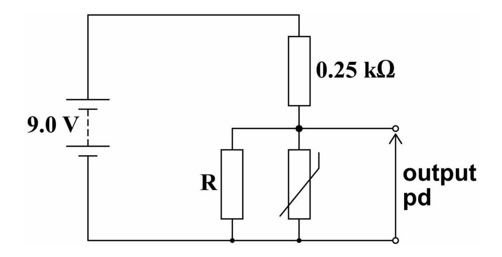
The supply has negligible internal resistance and the thermistor has a resistance of  $750~\Omega$  at room temperature. The student wants the output potential difference (pd) at room temperature to be 5.0~V
