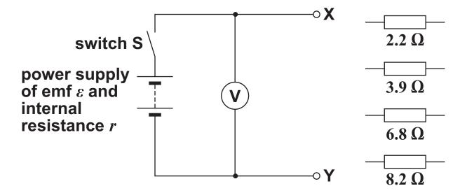
The student can change the external resistance R of the circuit between terminals X and Y. This is done by connecting different combinations of TWO resistors in series or in parallel between X and Y. This method can produce 12 DIFFERENT VALUES for R.
