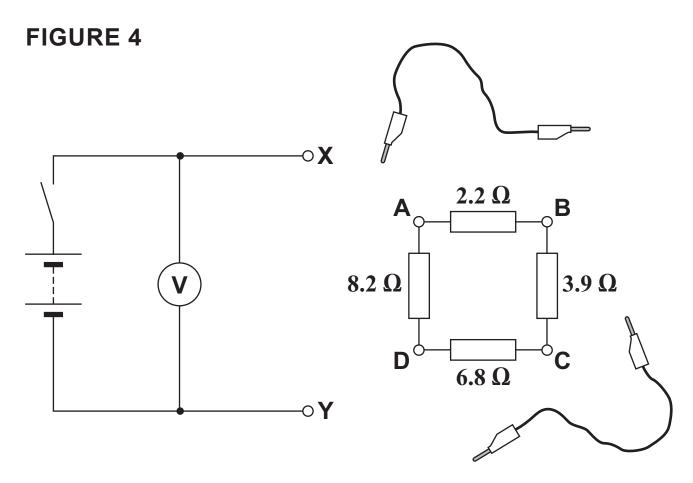
The four resistors are connected in a loop with sockets A, B, C and D at each junction. Two leads are used to connect the resistor loop to X and Y.
