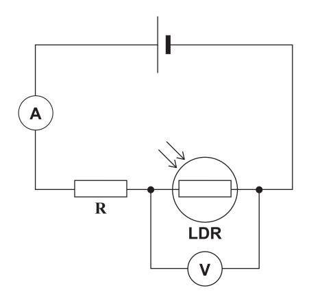
Which row shows how the readings on the ammeter and the voltmeter change when the light intensity incident on the LDR is increased? [1 mark]
