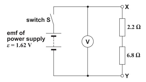
When S is closed the voltmeter reading V is 1·14 V.
