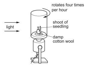
The platform was allowed to rotate for two days. It was left stationary for a further two days.
