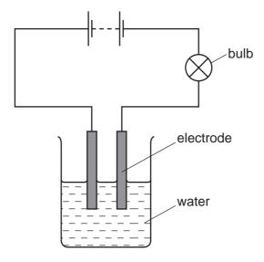
After the student adds substance **X** to the water, the bulb lights.
