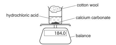
The beaker was placed on a balance and the mass of the beaker and contents recorded every minute.
