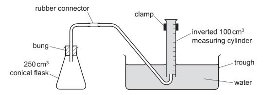
The trough should be large enough to allow the measuring cylinder to be filled with water in the trough.
