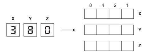
(c) If any of the 4-bit binary registers X, Y or Z contain the value 1 1 1 1 this indicates an error.
