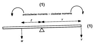
weight  $W \times \text{distance } Z = \text{weight } V \times \text{distance } Y$  (1)
