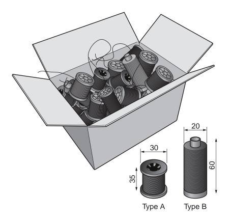
Design a storage system to house a selection of cotton reels when not being used. The system should hold at least 15 reels of Type A and 20 reels of Type B. All reels have an 8 diameter hole running through the centre.
