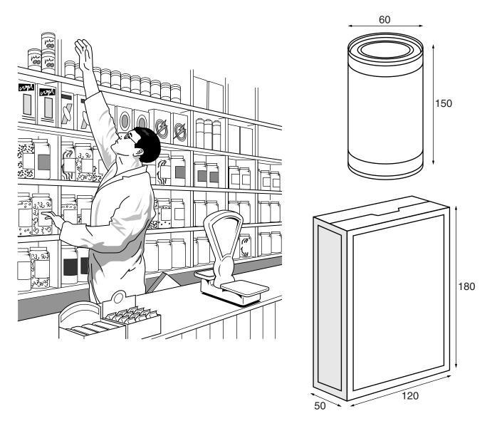
Design a device that would help the shopkeeper to reach and remove cans and packets of the types shown.
