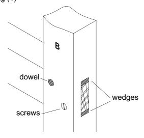
(iii) Temporary method could be screws, nails, G cramp, coach bolt. Allow other valid methods.
