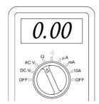
(iv) The reading should be less than  $1\Omega$ , 1 mark, allow buzzer may sound, 1 mark. [1]
