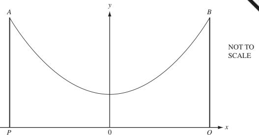
The diagram shows two vertical poles (AP and BQ) that support the ends (A and B) of a hanging chain.
