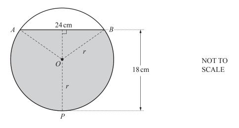
The diagram shows the cross section of a cylinder, center O, radius r, lying on its side. The cylinder contains water to a depth of 18 cm. The width, AB, of the surface of the water is 24 cm.
