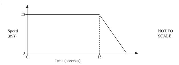
A car travels at  $20\,\text{m/s}$  for 15 seconds before it comes to rest by decelerating at  $2.5\,\text{m/s}^2$ .
