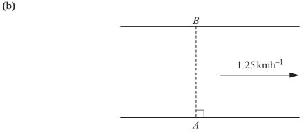
A river flows between parallel banks at a speed of  $1.25 \text{ kmh}^{-1}$ . A boy standing at point *A* on one bank sends a toy boat across the river to his father standing directly opposite at point *B*. The toy boat, which can travel at  $v \text{ kmh}^{-1}$  in still water, crosses the river with resultant speed 2.73 kmh<sup>-1</sup> along the line *AB*.
