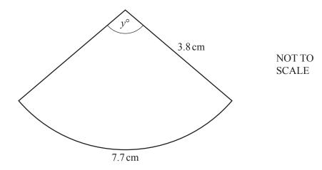
The diagram shows a sector of a circle of radius  $3.8\,\mathrm{cm}$ . The arc length is  $7.7\,\mathrm{cm}$ .
