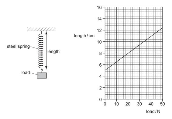
What is the extension of the spring when a load of 20 N is applied to it?
