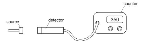
The reading on the counter shows how much radiation is reaching the detector.
