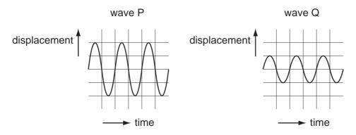
How do the frequency and pitch of P compare with the frequency and pitch of Q?
