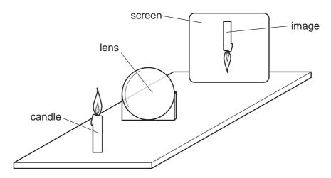
Various focused images are produced on the screen by moving the lens and the screen backwards and forwards.
