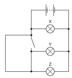
Which lamps are on and which lamps are off?
