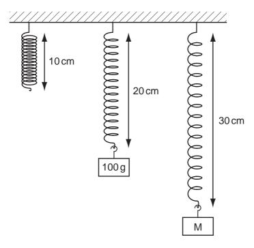
The extension of the spring is directly proportional to the mass hung on it.
