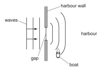
What is the name of this curving effect, and how can the gap be changed so that the waves are less likely to reach the boat?
