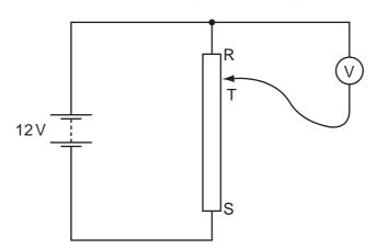
What happens to the reading on the voltmeter as the sliding terminal T is moved from R to S?
