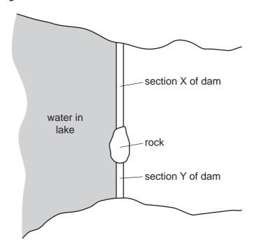
The water creates a force on each section of the dam and a pressure on each section of the dam.
