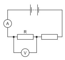
The reading on the ammeter is 2.0 A and the reading on the voltmeter is 8.0 V.
