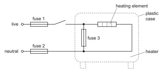
Which of the fuses are correctly placed?
