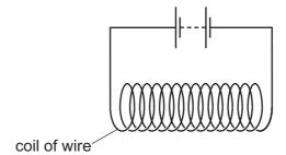
Which diagram shows the shape of the magnetic field produced in the middle of the coil?
