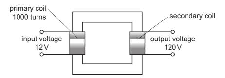
How many turns are on the secondary coil of the transformer?
