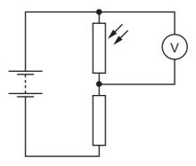
The brightness of the light falling on the LDR is increased.
