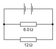
What could be the combined resistance of this arrangement of resistors?
