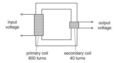
The input voltage is 240 V.
