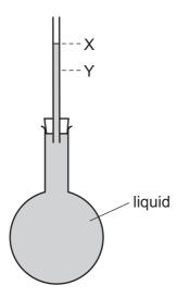
The flask is now placed in ice, and the liquid level in the tube falls to level Y.
