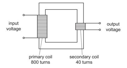
The input voltage is 240 V.
