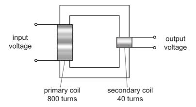
The input voltage is 240 V.
