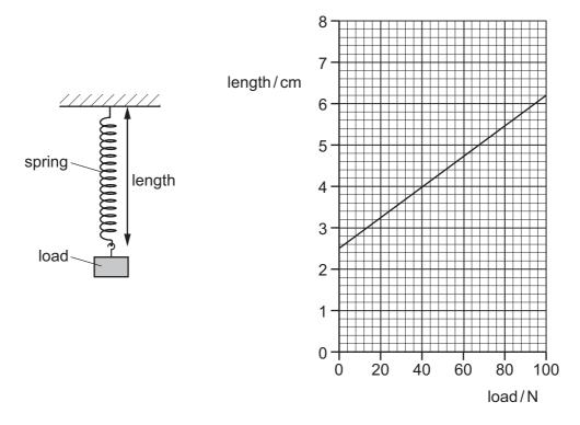
What is the extension of the spring when a load of 40 N is applied to it?
