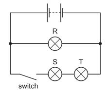
When the switch is open, which lamp or lamps are not lit?
