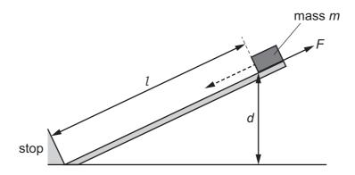
As the box slides down the slope, it loses gravitational potential energy and it does work against the friction.
