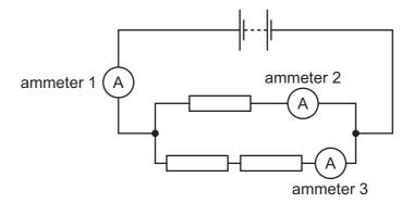
What is the order of the magnitudes of the readings on the ammeters from smallest to largest?
