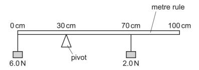
The rule balances when a weight of 6.0 N is hanging from the zero mark and a weight of 2.0 N is hanging from the 70 cm mark.
