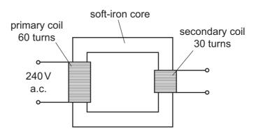
What is the potential difference across the secondary coil of the transformer?
