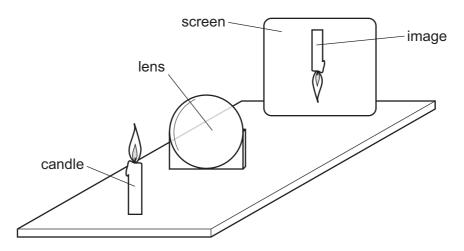
Various sharp images are produced on the screen by moving the lens and the screen backwards and forwards.
