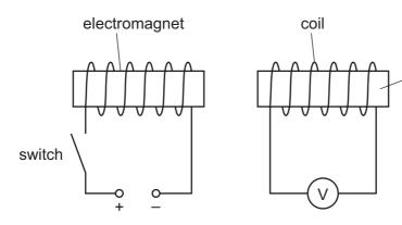
The switch is closed. The electromagnet magnetises quickly.
