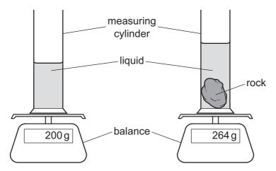
Which two measurements does the student need to make to determine the density of the rock?
