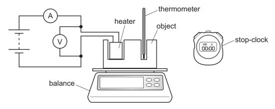
Which piece of apparatus could be omitted if the purpose of the experiment is to determine the thermal capacity of the object?
