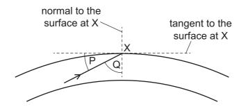
The light is totally reflected within the fibre.
