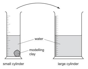
The reading on the small measuring cylinder goes down by 20 cm<sup>3</sup>.
