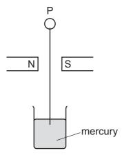
The wire is hanging vertically between the N and S poles of a magnet.
