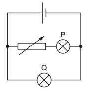
The resistance of the variable resistor is increased.
