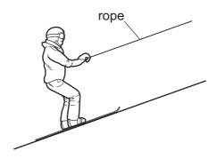
The tension in the rope is 100 N and there is a combined frictional and air resistance force of 20 N acting on the skier.
