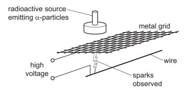
When the radioactive source is placed close to the grid, sparks are observed in the position indicated.
