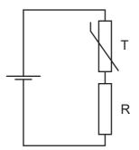
$V_{R}$  and  $V_{T}$  are the potential differences across R and T respectively.
