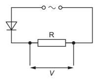
Which graph shows how the voltage V across the resistor R varies with time?
