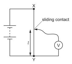
He changes the length of wire  $\it l$  by moving the sliding contact along the resistance wire.
