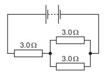
What is the combined resistance of the three resistors in this circuit?
