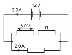
What is the current in resistor R and what is the p.d. across resistor R?
