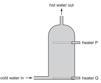
When only heater Q is switched on, it takes a very long time to heat the tank of water to the required temperature of 60 °C.
