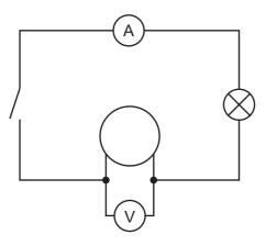
(ignore orange) to include ammeter in series and voltmeter in parallel, (allow two lamps OR two switches) correct symbols ;;
