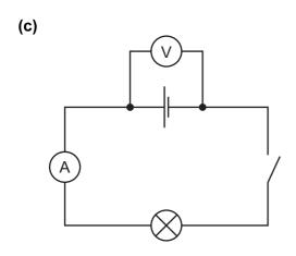
voltmeter connected correctly; ammeter connected correctly;
