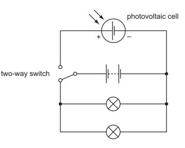
complete circuit and two lamp symbols; correct parallel arrangement;
