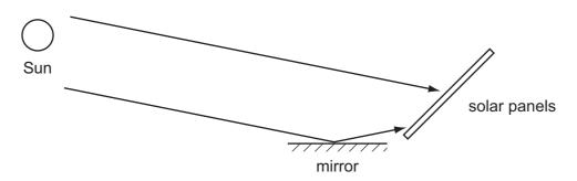
any direct ray + ray reflected from mirror to solar panel (both required); angle of incidence = angle of reflection; [2]
